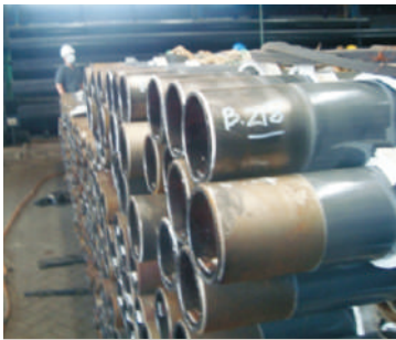
Fusion Bond Epoxy Coating (FBE)
